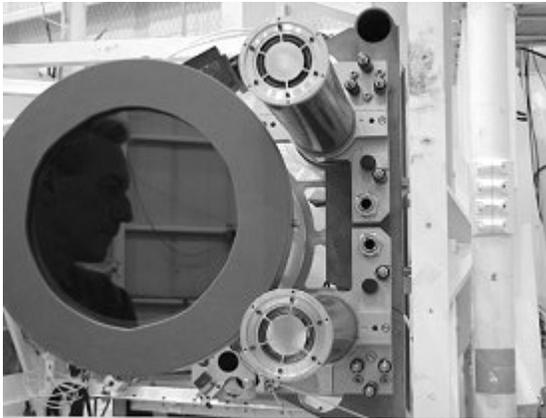
Earlier this year the team assembled a prototype double-barreled x-ray telescope consisting of two mirror assemblies with three shells each. It passed laboratory tests with flying colors, but that wasn't enough. An x-ray telescope on the ground is like an optical telescope with the lens cap on. "Cosmic x-rays don't reach Earth's surface," explains Ramsey, "because our atmosphere is opaque to this high energy radiation." It was time to go to space -- or as near to it as they could get.
