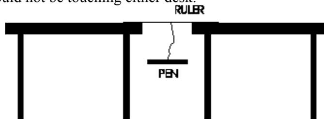
2. For the rest of this experiment if you are asked to charge a pen, hold it by its cap and rub it briskly 50 times with the piece of wool. If you are asked to discharge a pen, roll it gently between your hands a few times.
