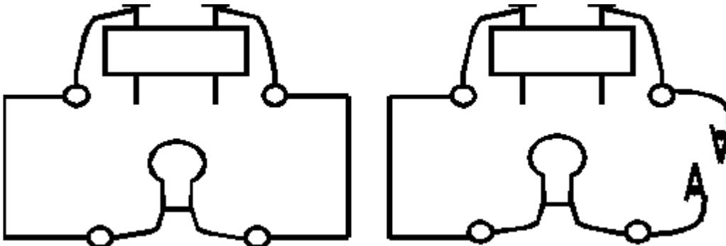
3. Complete the circuit by clipping each of the materials in the bag-o-stuff between the clips.
