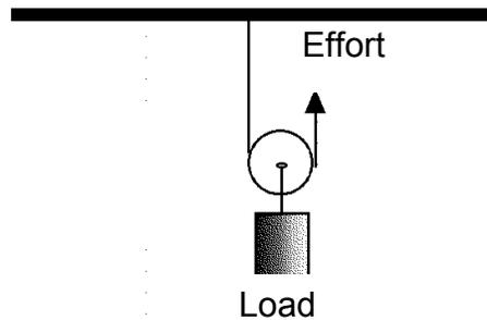
These two types of pulleys can be combined to form DOUBLE PULLEYS, which have at *least two wheels*. There are different combinations that can result in a double pulley. As the pulley becomes more complex, the total lifting effort decreases. For example, a system made of a fixed pulley and a movable pulley would reduce the workload by a factor of two, because the two pulleys combine to lift the load.
