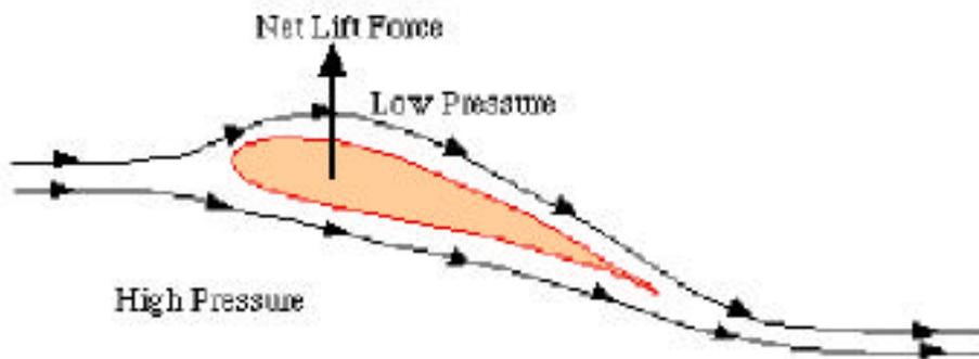
A difference in pressure causes the lifting force
